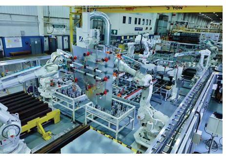
Shiloh's laserwelding process produces aluminum blanks for stamping. the trend of lightweighting to continue and we want to be the primary metal of choice when it comes to our customers and designing lightweight vehicles."
